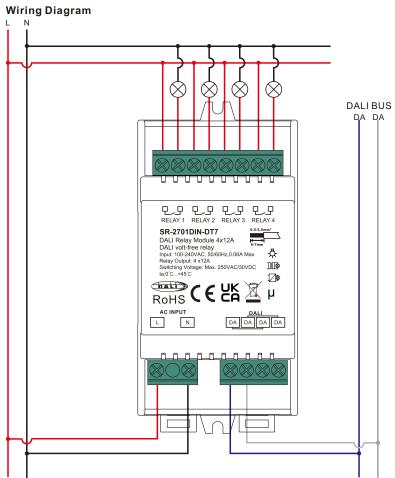
Note: please use 2.5mm² wire for relay in and out connections, small size wire will cause over heating.
